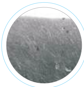
TiAlN base multi-elements coating (YBG105)
