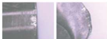
ZCC-CT insert after 80 minutes machining
