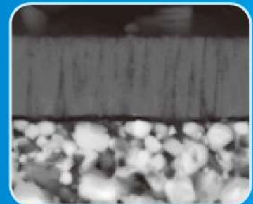
PVD coating organization structure of cermet
